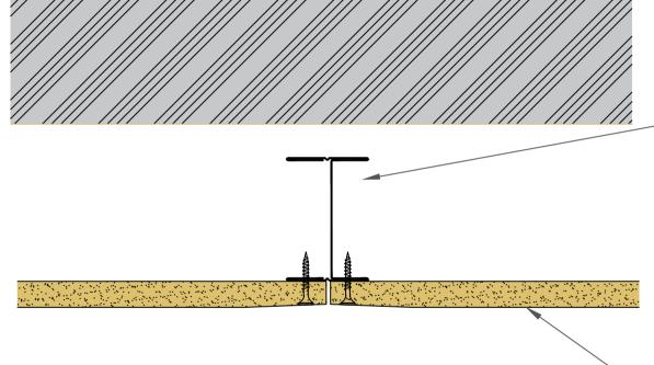
SPEEDLINE 60mm 'I' Studs at 600mm Ctrs
